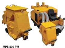
The MPB 500 PW attachment uses a different concept to conventional wheel blast equipment. Using a 400mm (15.7") wide machined drum with L shaped manganese blades attached, the the process works with a similar principle to a paddle steam boat throwing abrasive at the surface in a uniform pattern across the width of the blast. The blast pattern fades at the edges, eliminating "tram lines" from one pass to the next, ensuring this attachment is ideal for cleaning or preparing large surface areas.
